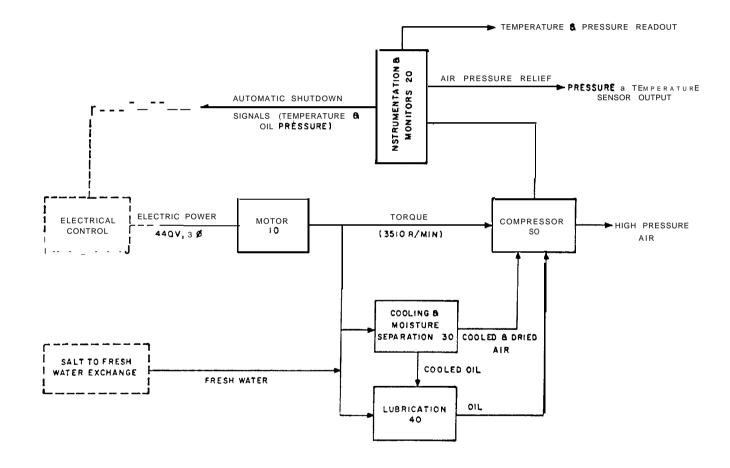
Figure 101.1 Example of a functional block diagram
