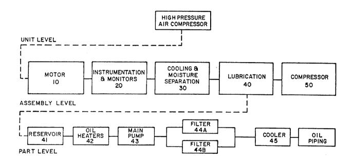
Figure 101.2 Example of a reliability block diagram
